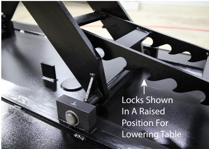
Note: When lift is not in fully lowered position, it is recommended that the nearest lock position be used.
